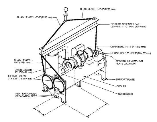
\*Carrier recommends that "I" Beam Spreader Bars be field supplied and installed. NOTES:
